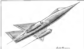
TOMORROW'S DAY FIGHTER probably will have delta wing, variable area, lightweight jet, integral construction
